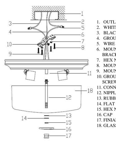
1. OUTLET BOX WHITE WIRE 3. BLACK WIRE 4. GROUND WIRE 5. WIRE CONNECTOR 6. MOUNTING BRACKET 7. HEX NUT 8. MOUNTING SCREW 9. MOUNTING SCREW **10. GROUND WIRE SCREW 11. CONNECTOR** 12. NIPPLE **13. RUBBER WASHER** 14. FLAT WASHER 15. HEX NUT 17. FINIAL 18. GLASS
